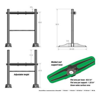
MAPA Products Supports are designed and manufactured in accordance with MSS SP-58-2002 and MSS SP-69-2002.
